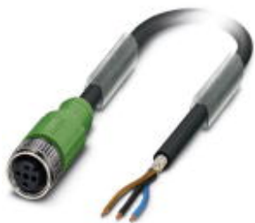
Sensor/actuator cable, 3-position, Variable cable type, shielded, free cable end, on Socket straight M12, A-coded, cable length: Free input (0.2 ... 40.0 m)
