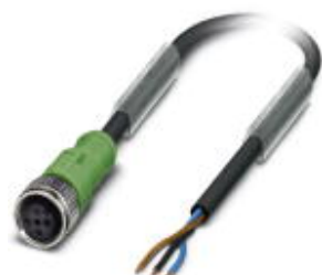
Sensor/actuator cable, 3-position, PUR halogen-free, black-gray RAL 7021, free cable end, on Socket straight M12, A-coded, cable length: 10 m
