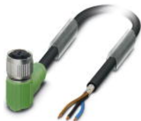
Sensor/actuator cable, 3-position, Variable cable type, shielded, free cable end, on Socket angled M12 SPEEDCON, A-coded, cable length: Free input (0.2 ... 40.0 m)
