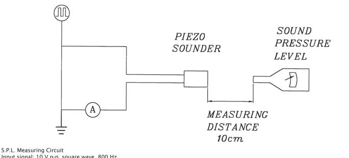
Input signal: 10 V p-p, square wave, 800 Hz Mic: RION S.P.L. meter UC30 or equivalent S.G.: Hewlett Packard 33120A function generator or equivalent
