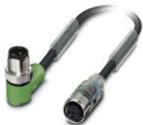
Sensor/actuator cable, 3-position, Variable cable type, Plug angled M12 SPEEDCON, A-coded, on Socket straight M12 SPEEDCON, A-coded, with 2 LEDs, cable length: Free input (0.2 ... 40.0 m)
