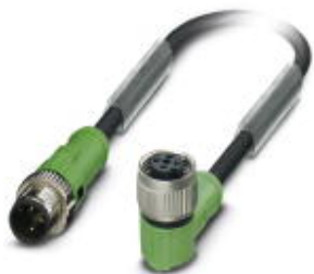
Sensor/actuator cable, 3-position, Variable cable type, Plug straight M12 SPEEDCON, A-coded, on Socket angled M12 SPEEDCON, A-coded, PIN 2+4 bridged, cable length: Free input (0.2 ... 40.0 m)
