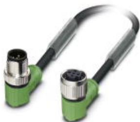
Sensor/actuator cable, 5-position, Variable cable type, Plug angled M12 SPEEDCON, A-coded, on Socket angled M12 SPEEDCON, A-coded, cable length: Free input (0.2 ... 40.0 m)
