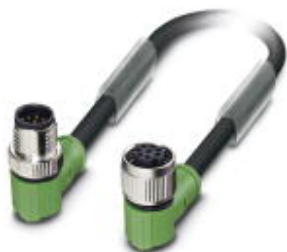
Sensor/actuator cable, 8-position, Variable cable type, Plug angled M12 SPEEDCON, A-coded, on Socket angled M12 SPEEDCON, A-coded, cable length: Free input (0.2 ... 40.0 m)
