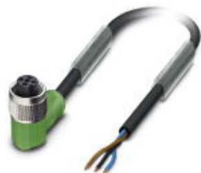
Sensor/actuator cable, 3-position, Variable cable type, free cable end, on Socket angled M12, A-coded, cable length: Free input (0.2 ... 40.0 m)
