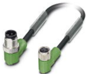
Sensor/actuator cable, 3-position, Variable cable type, Plug angled M12, A-coded, on Socket angled M8, cable length: Free input (0.2 ... 40.0 m)
