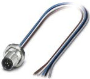
Sensor/actuator flush-type plug, 5-pos., M12, A-coded, rear/screw mounting with Pg9 thread, with 0.5 m TPE litz wire, 5 x 0.34 mm², stainless steel version
