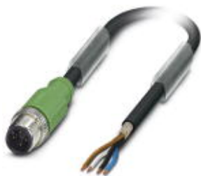
Sensor/actuator cable, 4-position, PUR halogen-free, black-gray RAL 7021, shielded, Plug straight M12, A-coded, on free cable end, cable length: 3 m
