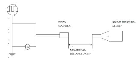
Mic: RION S.P.L meter UC30 or equivalent Mic: TION UC30 S.G: Hewlett Packard 33120A Function Generator or equivalent S.G: Hewlett Packard 33120A
