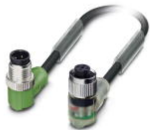
Sensor/actuator cable, 4-position, Variable cable type, Plug angled M12, A-coded, on Socket angled M12, A-coded, with 3 LEDs, cable length: Free input (0.2 ... 40.0 m)
