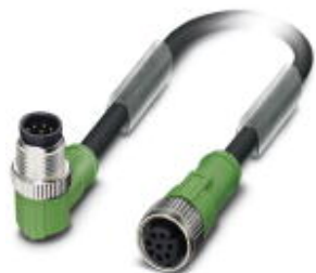
Sensor/actuator cable, 8-position, Variable cable type, Plug angled M12, A-coded, on Socket straight M12, A-coded, cable length: Free input (0.2 ... 40.0 m)
