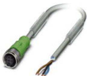
Sensor/actuator cable, 4-position, PUR halogen-free, highly flexible, gray RAL 7001, free cable end, on Socket straight M12, A-coded, cable length: 5 m, for robots and drag chains
