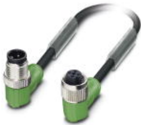
Sensor/actuator cable, 3-position, Variable cable type, Plug angled M12, A-coded, on Socket angled M12, A-coded, PIN 2+4 bridged, cable length: Free input (0.2 ... 40.0 m)
