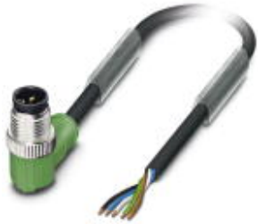
Sensor/actuator cable, 5-position, PUR halogen-free, black-gray RAL 7021, Plug angled M12, A-coded, on free cable end, cable length: 1.5 m
