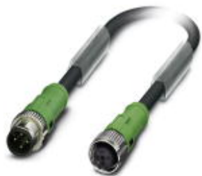
Sensor/actuator cable, 4-position, PUR, black-gray RAL 7021, Plug straight M12 SPEEDCON, A-coded, on Socket straight M12 SPEEDCON, A-coded, cable length: 2 m
