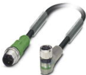
Sensor/actuator cable, 3-position, PUR halogen-free, black-gray RAL 7021, Plug straight M12, A-coded, on Socket angled M8, with 2 LEDs, cable length: 5 m
